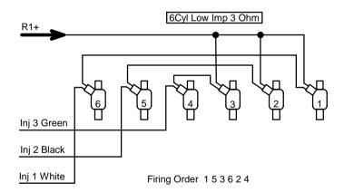
**Note!** Your firing order and piston numbers may differ from the examples. Determine which pistons move up and down together and wire them together. See also the manual for how to determine from the firing order which injectors must be grouped together.
