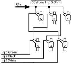
**NB!** Connect the Positive to the Negative between injectors
